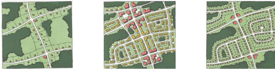
Block structure for the following residential land use categories: very low density, low density, and medium density.
